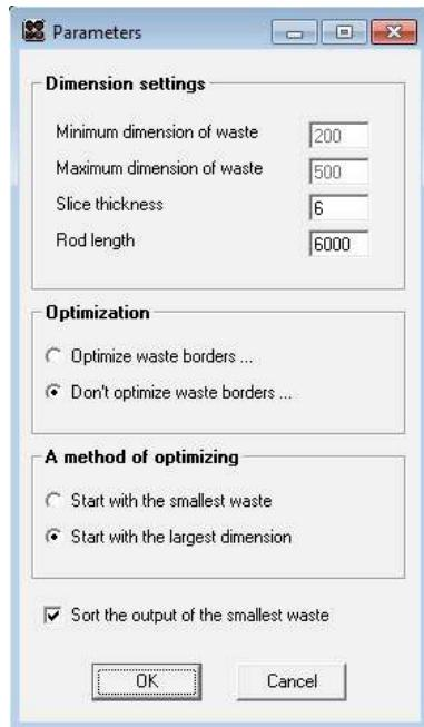
In **Dimension setting** first select the length of the rod in mm. This is the material from which you cut (default 6000 mm). Select slice thickness (default 6 mm).
